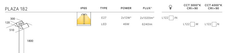
Complies with UNI 10819 on the limitation of the dispersion upwards of the luminous flux.
